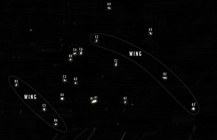
This mosaic shows images of the same star. Each is labeled with the name of the mirror segment that captured it. "Wing" refers to the two sides of the mirror assembly that unfolded in space. (Source: NASA)
