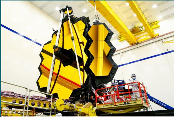
Folding mirror segments for the James Webb Space Telescope on Earth. Northrop Grumann
