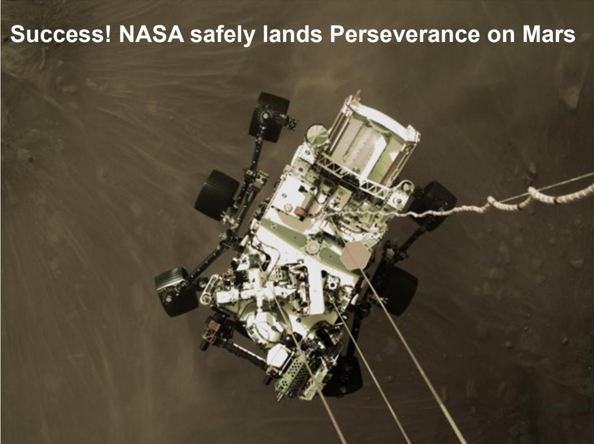
Perseverance captured video of its entire landing stage. This still image shows the rover being lowered down to Mars' surface via its Skycrane maneuver.
